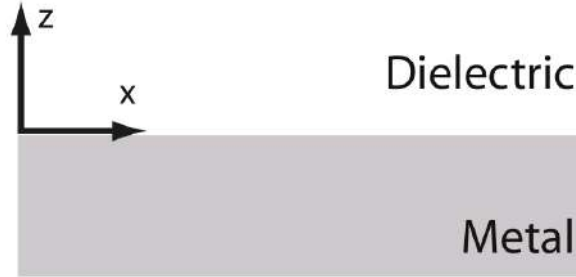
Fig. 4 Geometry of the surface plasmon-polariton propagation at an interface between a dielectric and a metal.
